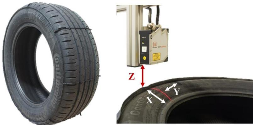
**Fig. 1.** The scanned object and detail of the selected area during the scanning process.
