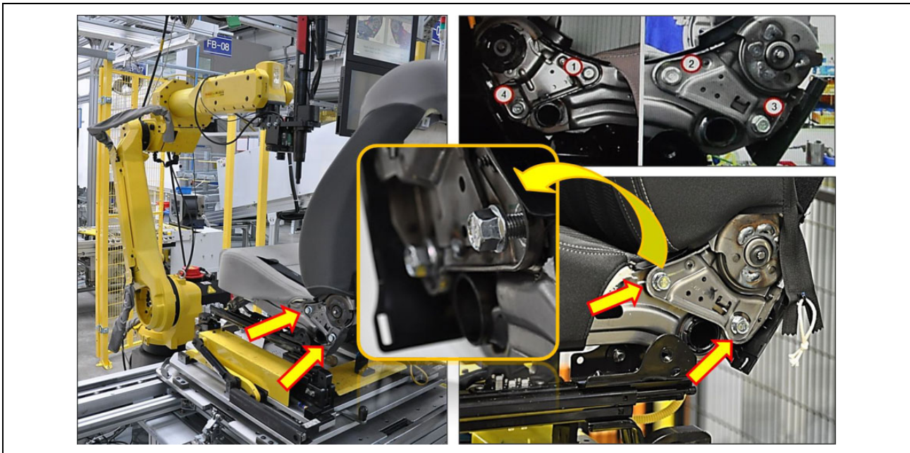
Figure 1. The Bolting station definition—basic structure of the workcell (left), detail of scanned area for finding of screws (right down), screwing order definition (right up), and detail on prescrewed bolt in position how is entering the station (middle).
