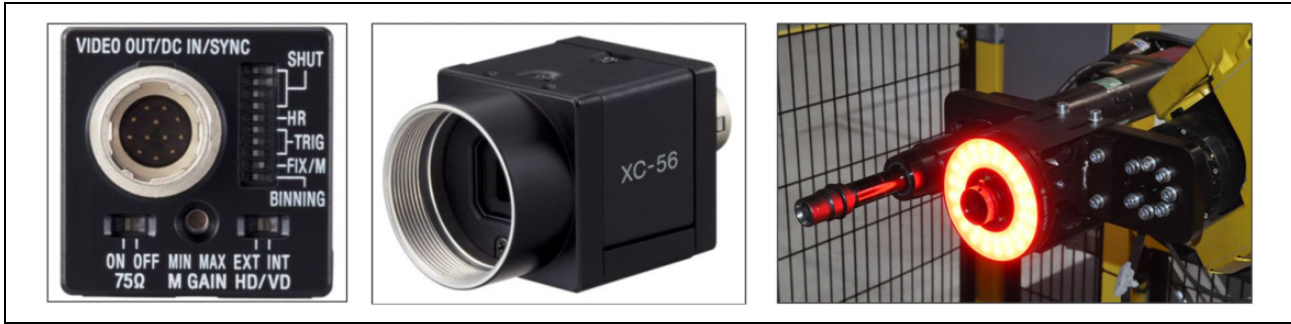
Figure 4. Camera Sony XC-56—rear and front view (left/middle) and its mounting on common holder with the screwdriver (right).
