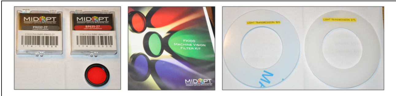
Figure 6. Tested filtering elements—light red bandpass filter BP635-27 and linear polarizer PR032-27 and diffuser rings with different light transmission level.
